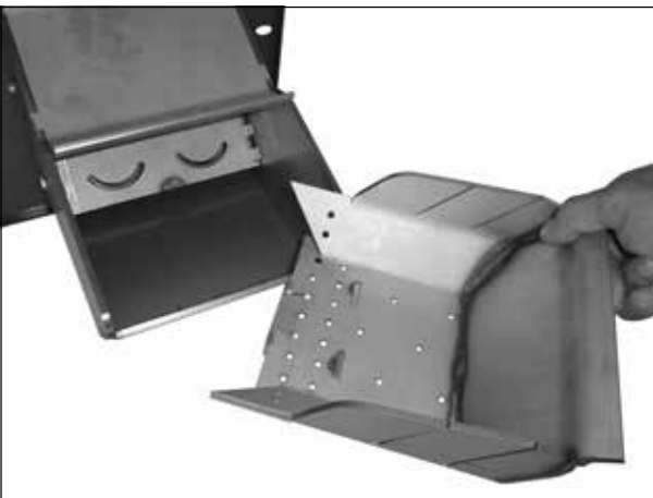
Removable combustion chamber - must be regularly cleaned
