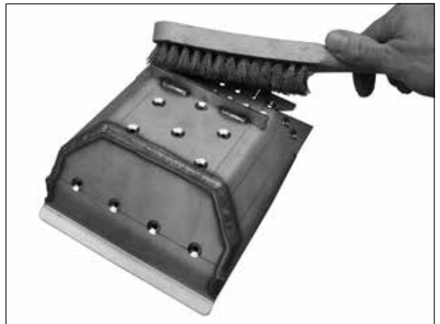
Demonstration of cleaning the combustion chamber
