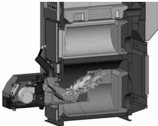
Burner flame ending 1 - 3 cm before the opposite wall
